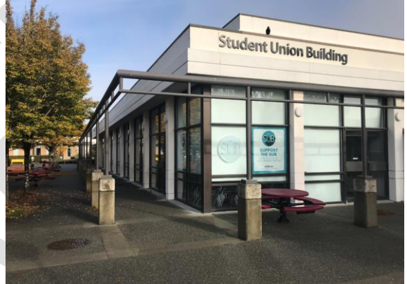
Photo 6.8 – 1996 addition, Visible Kawneer storefront glazing with steel frame in front to accommodate exterior shading devices.
